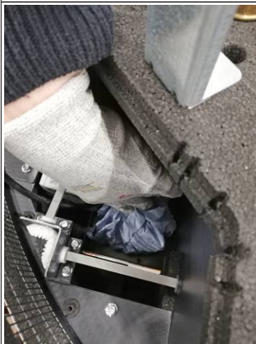
Fig. 34: Cleaning the pump sump
