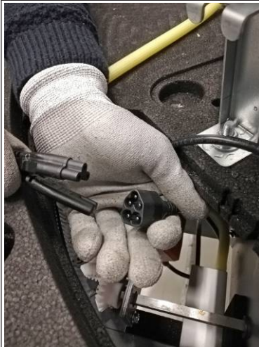
Fig. 33: Loosening the cable
