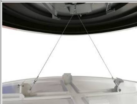
Fig. 28: Base plate safety cables
